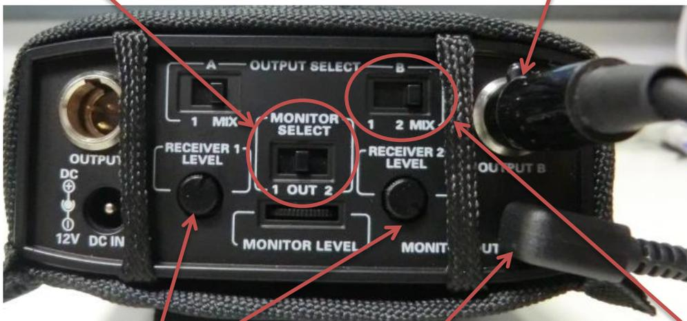
The recording volume of the 2 microphones can be adjusted using the Receiver 1 and 2 Level dials (eg. to give dominance to academic feedback).
