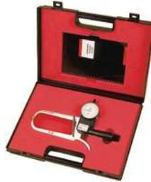
**When taking measurements, do not allow the calipers to snap shut onto the test subject, as this could cause discomfort and cause damage to the indicator mechanism.**
